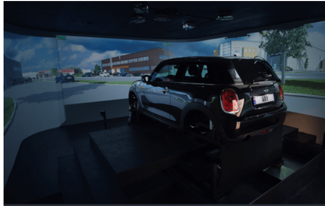
Figure 1: High-fidelity traffic simulator developed at Way AS. A real car is mounted on the motion platform in the center. Surrounding the car is a projection screen wall with six different view channels projected at the driver's front.
