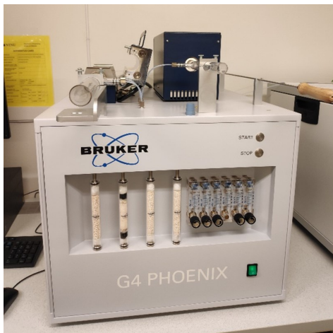
Figure 3.11: Image of the Bruker G4 Phoenix that was used for hot extraction.
