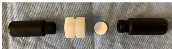
FIGURE 2 Left: sample vial, support membrane union, circular support membrane and acceptor vial; right: 10-position holder with 1 extraction cell.
