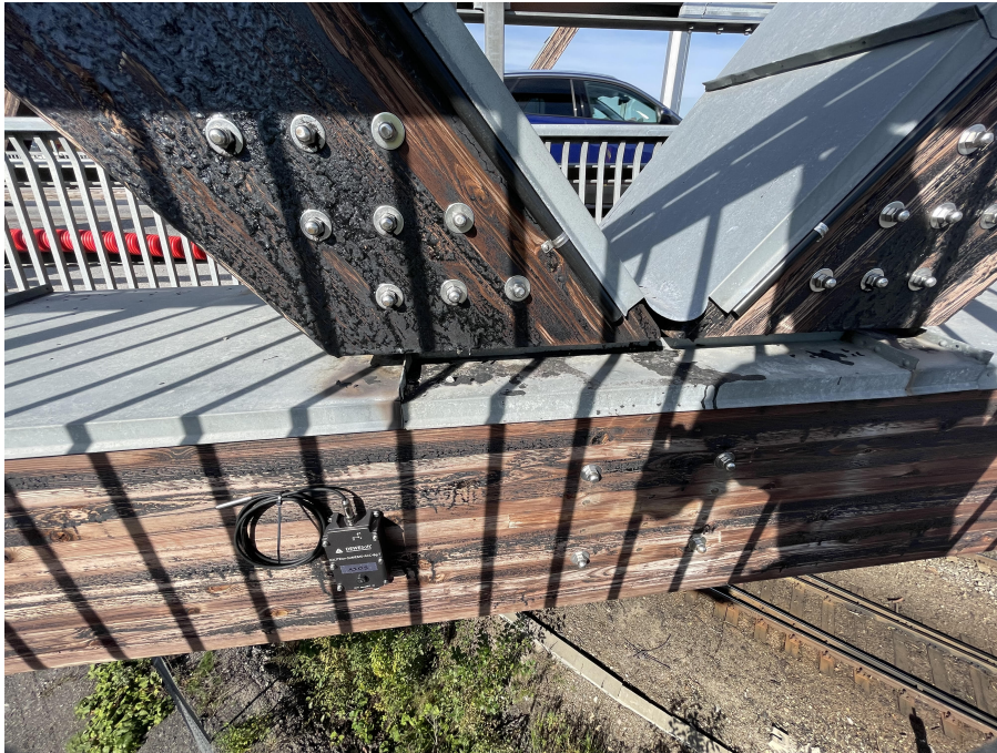
Figure 10: Example of the distance between the center of the junction to the location of the accelerometer.
