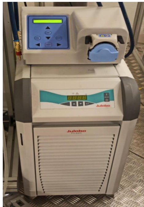
Figure 32: Chilling unit for condenser.
