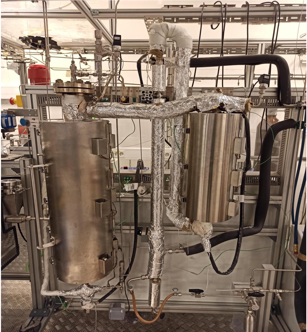
Figure 40: Biomass to aviation fuel pilot plant without gas filter.
