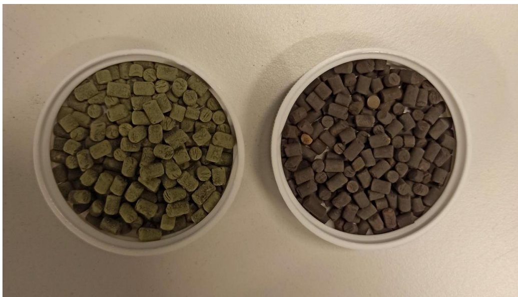
Figure 26: Fresh (left) and spent (right) catalyst prepared inhouse.
