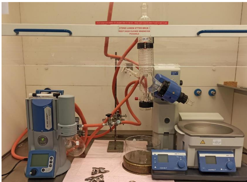
Figure 25: Rotary evaporator setup for bio-oil separation.
