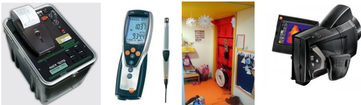
Figure 3. Devices used for measurement: RAD 7 (left), Testo 435-2 (middle-left), Minneapolis Blower Door (middle right), Testo 885-2 (right)
