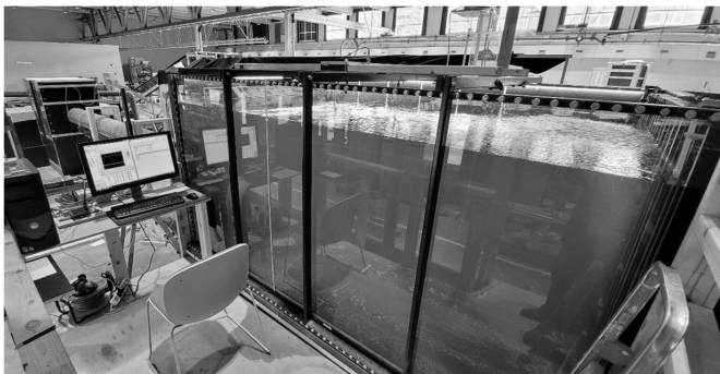
Fig. 5. Physical culvert model, showing head tank, barrel, tailwater tank, and data station. (Image by Elena Pummer.)
