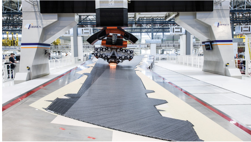
Figure 2.2.1: Layup of a composite wing skin using AFP (Airbus A350) [44].
