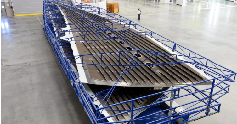
Figure 1.3.2: Composite lower wing skin panel (Airbus A350) with access holes distributed along the spanwise direction [27].
