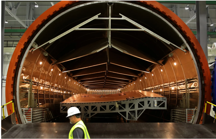
Figure 2.2.3: Autoclave cure of a composite wing skin (Airbus 777X) [46].
