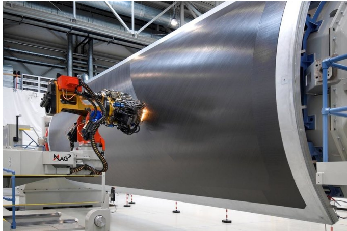
Figure 1.1.1: Manufacturing of a composite fuselage section (Airbus A350) with fibers being placed on the mandrel in linear paths [7].
