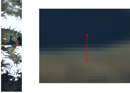
(a) Selected edge of an image acquisition. The edge response along the red dashed line is shown in the next subfigure.
