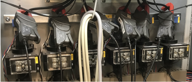
Fig. 3-8. Current probes used to to measure the six phase currents in the network
