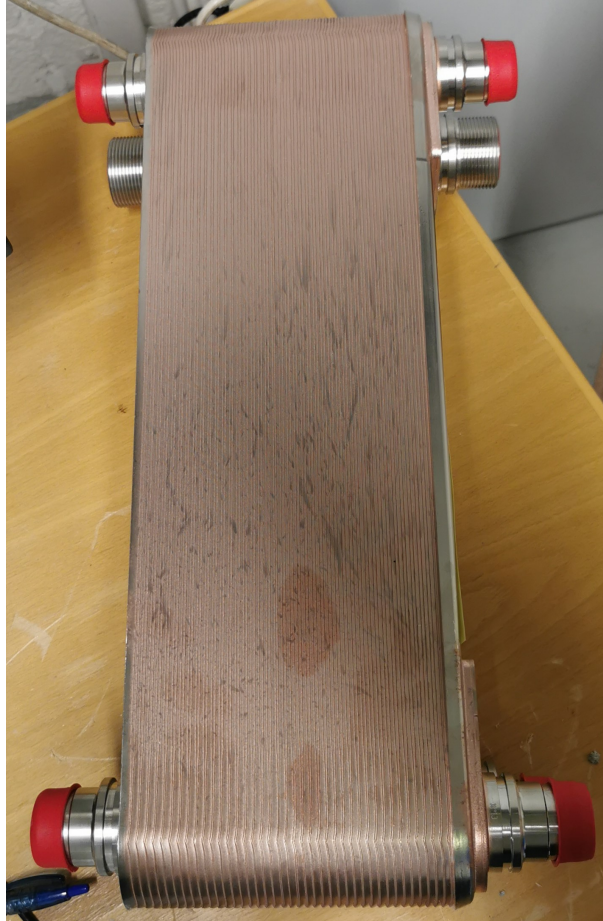
Figure 17: The two-stage evaporator before installation
