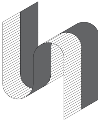
Figure 3: Flexible adhesive sealing strip. Note the adhesive on alternate sides of the strip.
