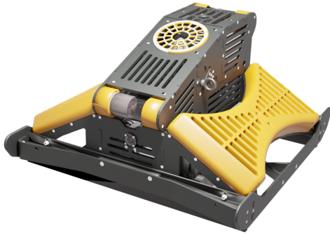
Fig. 1: The Remora net cleaning robot. Image courtesy of Mithal AS [8].
