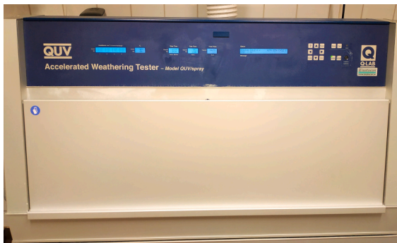
Fig. 2. Accelerated weathering tester (Model QUV/Spray).
