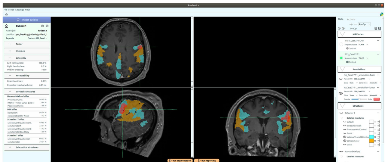
Figure 1. Illustration of the raidionics software GUI in single patient mode, after generating the standardized report over a glioblastoma case. The left side presents the tumor characteristics belonging to the report, the central part offers a set of 2D views, and the right panel shows loaded MR scans and corresponding annotations.
