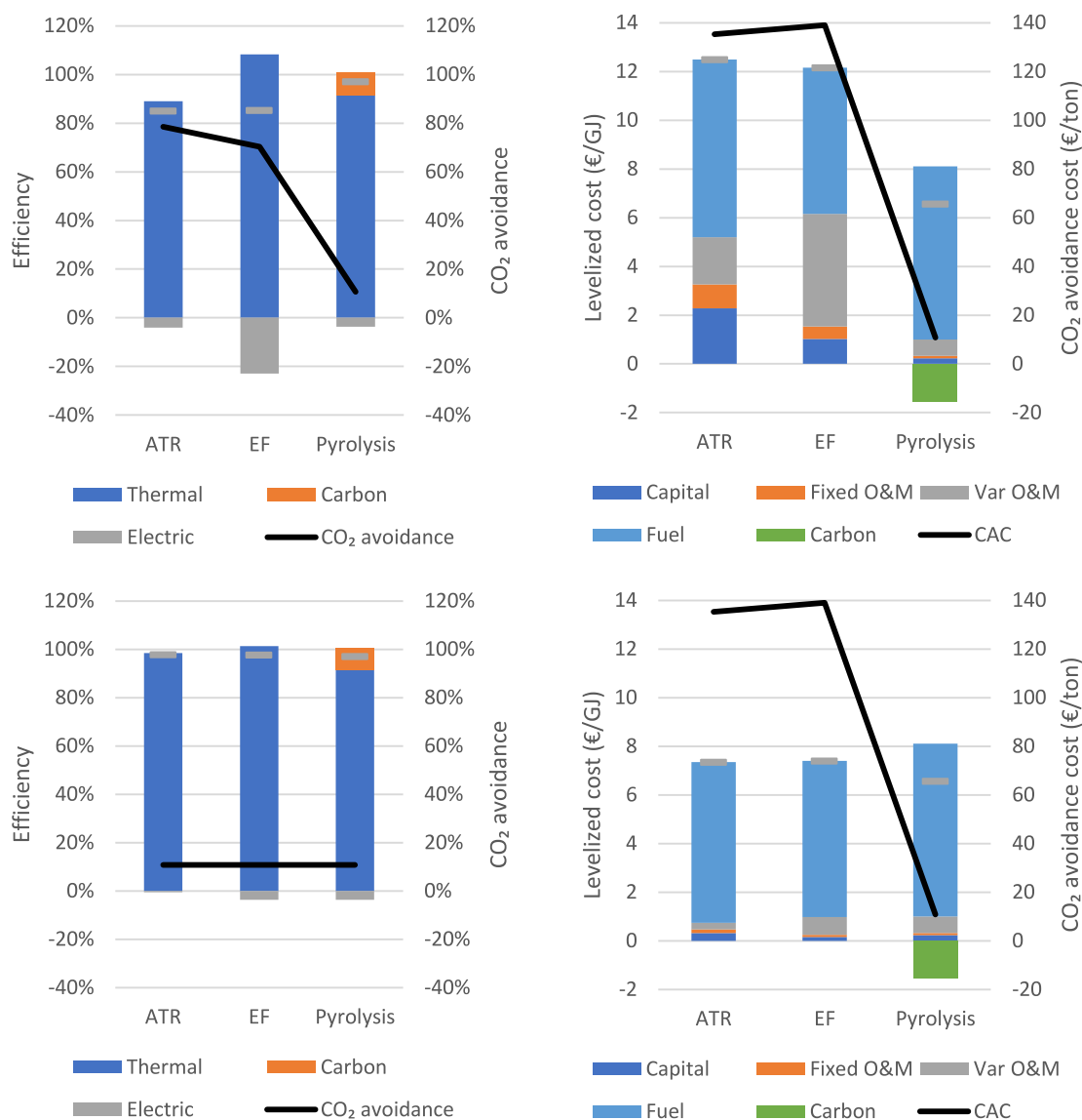
Fig. 4. Benchmarking of pyrolysis targeting 20% H 2 in the product stream at 800 °C reactor temperature against ATR and ER alternatives. Variable O&M costs consist mainly of electricity imports and the grey dashes indicate the summation of the different components of efficiency and levelized cost. Top row: Unadjusted results. Bottom row: Natural gas added to benchmark technologies to yield the same CO 2 intensity as the pyrolysis technology.
