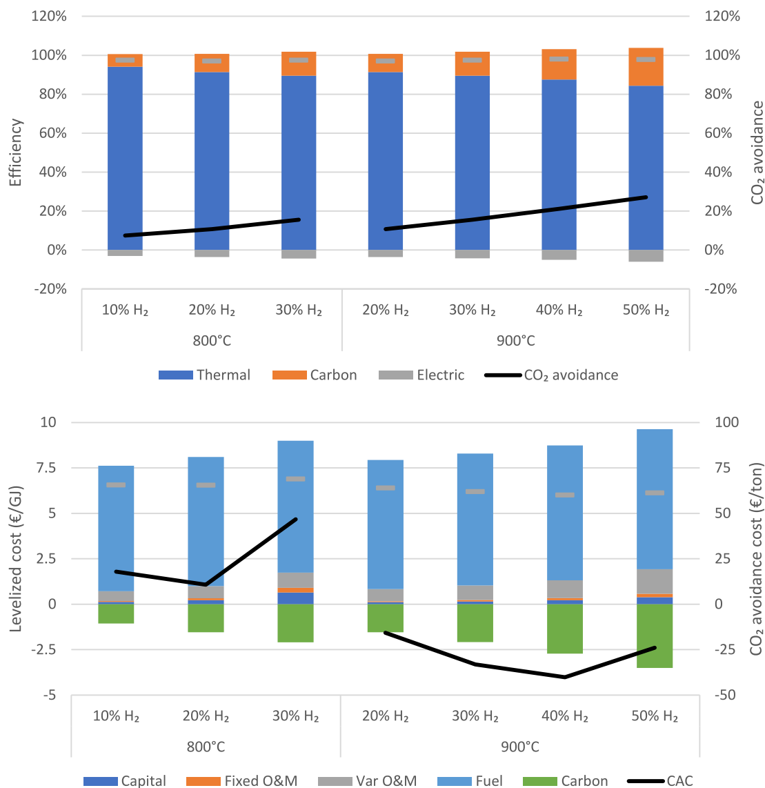
Fig. 6. The performance of the pyrolysis technology when delivering different H 2 fractions (higher fractions imply a closer approach to equilibrium requiring larger reactors) at reactor temperatures of 800 and 900 °C.
