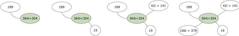
Figure 3.4: Drawing the 3-isogeny graph edge by edge by computing 3-isogenies from our starting curve with j -invariant of 364 \cdot i + 304 .
