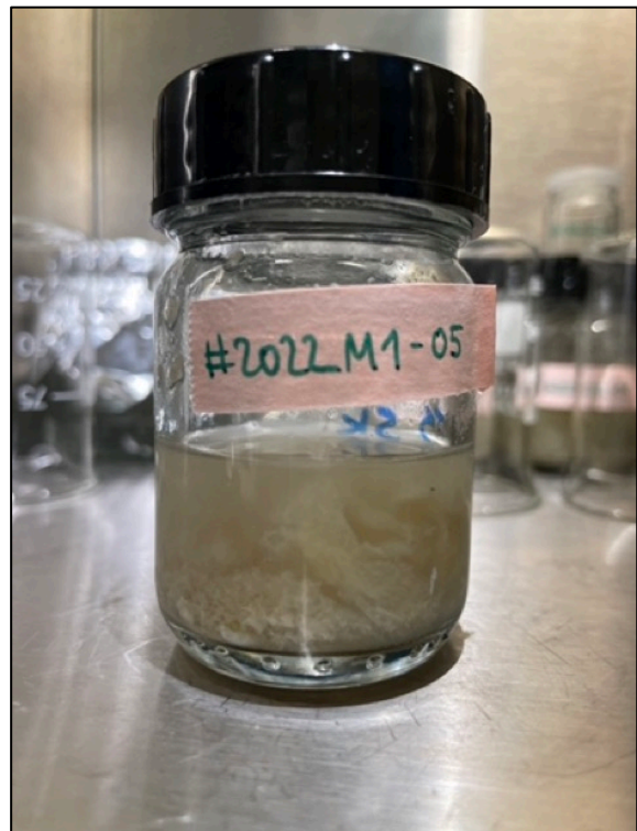
Figure D.2 – Step 1: Dissolving of pellet (b). Sample after 24h in ultrapure water on shaker table (175 rpm, 25°C). Slurry with loose otoliths.
