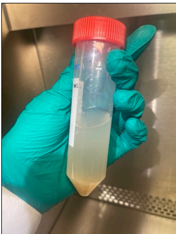
Figure D.11 – Step 3: Density separation (b). Sample after transfer to falcon tube and settling (1-2h, RT). The liquid removed to beaker \hat{=} supernatant 1 (S1).
