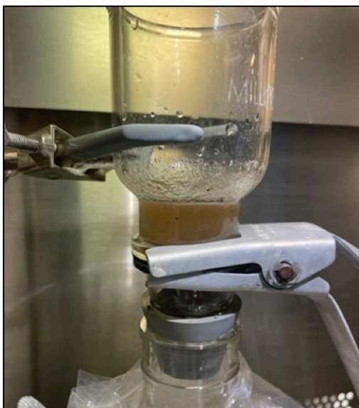
Figure 3.1 – A sample clogging the fine metal mesh filter (Photo: K. Buchholz)
