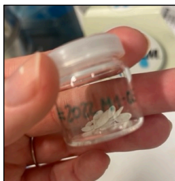
Figure D.4 – Step 1: Dissolving of pellet (d). Removed otoliths (thrice rinsed and then dried) in drams glass.
