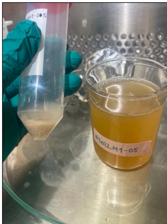
Figure D.10 – Step 3: Density separation (a). Sample after transfer to falcon tube and settling (1-2h, RT). The liquid removed to beaker \hat{=} supernatant 1 (S1).
