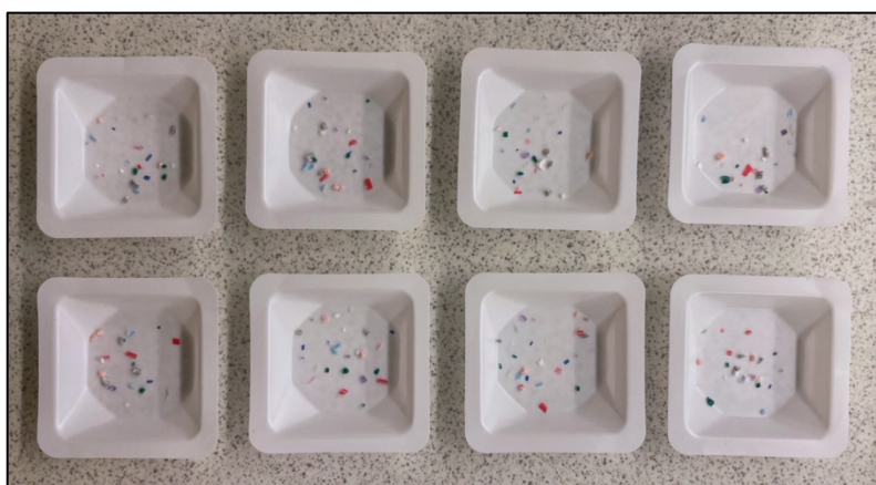
Figure 2.5 – Artificially created microplastic particles. These particles were cut from plastic collected on Sklinna during the field season of 2022. Each dish contains one batch of spikes. (Photo: K. Buchholz)
