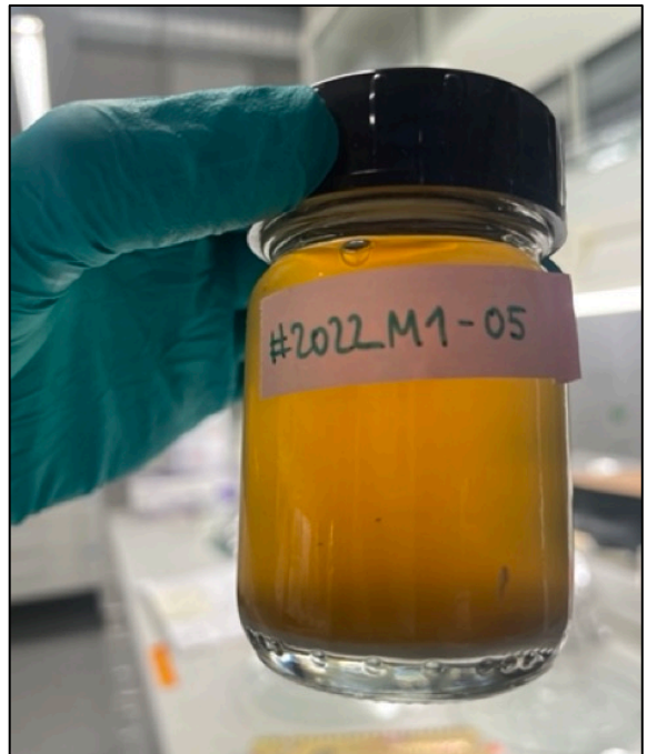
Figure D.8 – Step 2: Digestion of organic matter (d). Sample after 48h on shaker table (90 rpm, 40°C) in KOH solution. The detritus is more homogenous than at the previous stage.
