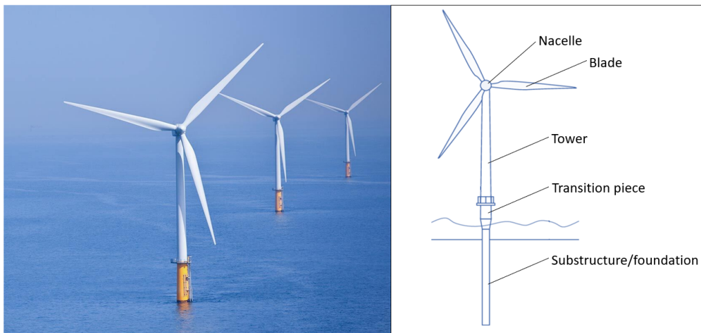
Figure 1: Offshore horizontal axis wind turbine (left). Offshore horizontal wind turbine sketch (right)
