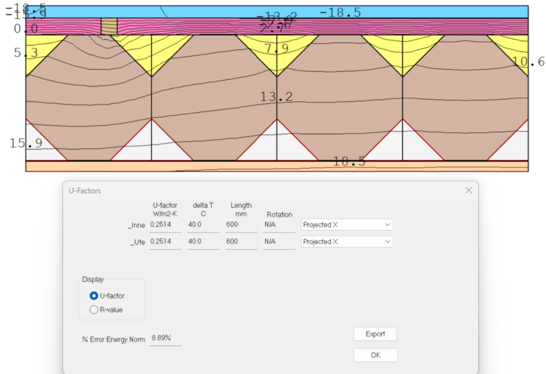
Figure C4: Excerpt from THERM that shows an illustration of the simulated wall and the results for Option 4 for simulation in THERM.
