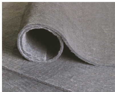
Figure 4.3: Spaceloft® Aerogel insulation blanket developed by Aspen Aerogels, Inc. (Glava AS, 2013).
