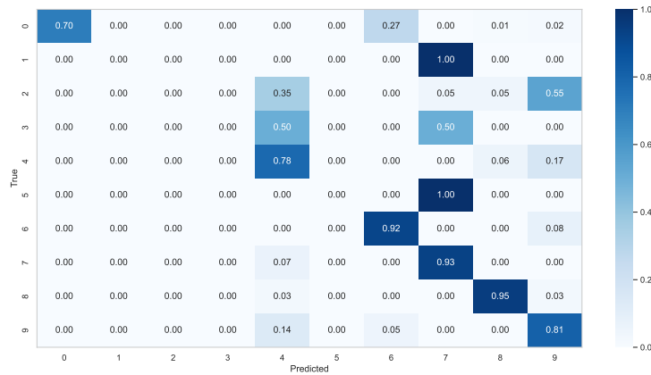
Figure 6.3: Confusion Matrix for classifier of the Inception architecture trained with IIC. Classes 1, 2, 3, and 5 are misclassified and underrepresented in the dataset.
