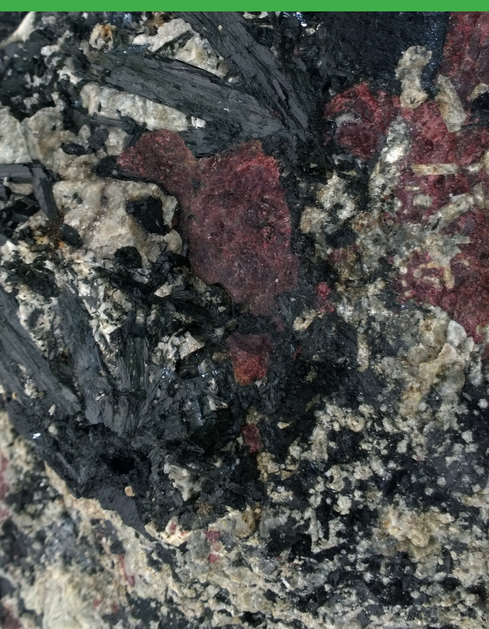
Pinkish HREE bearing Eudialite with black Arfvedsonite, Ilimaussaq complex, South Greenland (Credit: GKZ Freiberg)
