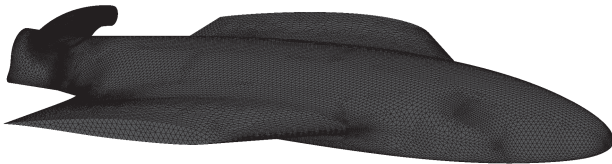
FIG 4. Geometry and Mesh of the PX-31 Falk used for the 3D simulation.
