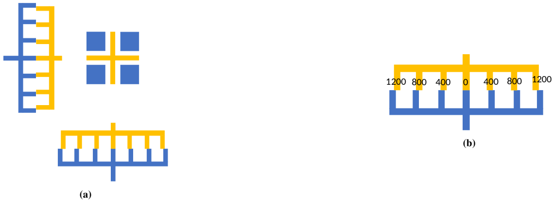
Figure 3.8: a) Common alignment mark in a multi-layer process. The two layers are represented by different colors. The cross is intended for coordinate reference, and the two calipers are used to measure the horizontal and vertical misalignment. b) Enlarged image of the caliper structures. The misalignment is measured by inspecting which of the branches align since they have a propagating displacement. The numbers are given in nm.
