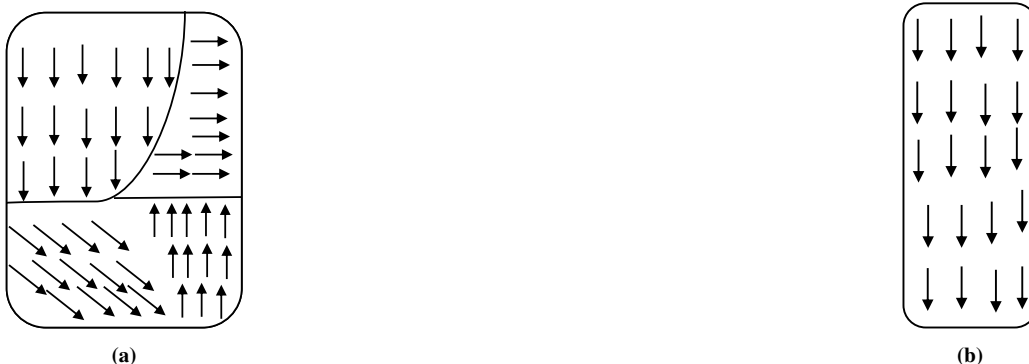
Figure 3.1: a) Ferromagnetic material with several domains. b) A single nanomagnet with uniform magnetization.
