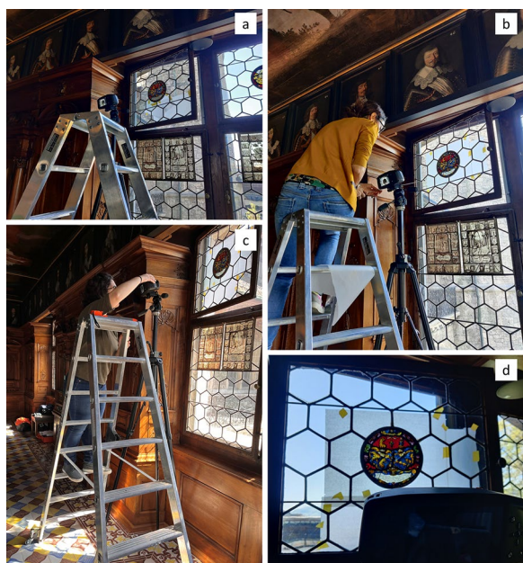
Fig. 3 Examples from the acquisitions of case studies IN-64.11; the diffusing sheet is placed on the glazing (historical window) behind the stained glass panel, so that it is not in touch with the artwork. In case of IN-64.11 the historical window was kept open to avoid having the tower (on the left side) within the field of view during the acquisition. For the other case studies the historical windows were closed after placing the diffusing sheet
