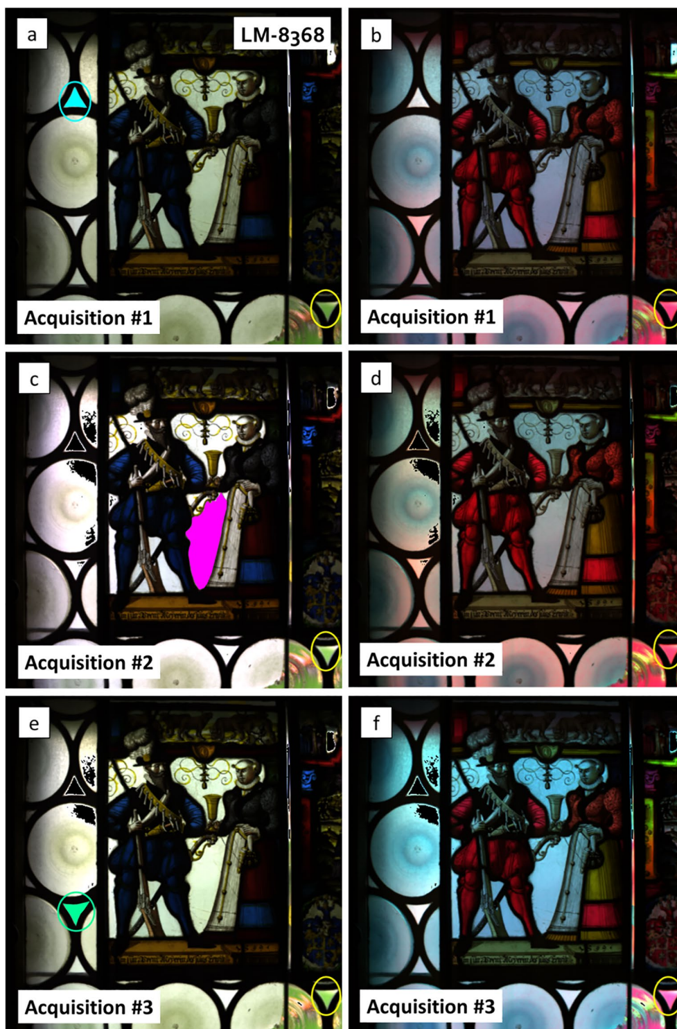
Fig. 12 a, c, e RGB images created by the camera after the acquisition, showing the area where the reference was collected (turquoise triangle for acquisition #1, magenta area for acquisition #2 and green triangle for acquisition #3); b, d, f false color images for each of the acquisitions. The band used to create the false color are stated in Fig. 13. The yellow circle indicates the area where the signal of vegetation (see Fig. 13) was taken. The black pixels visible in the small triangular glass pane and partially in the crown glass on the top left are saturated pixels
