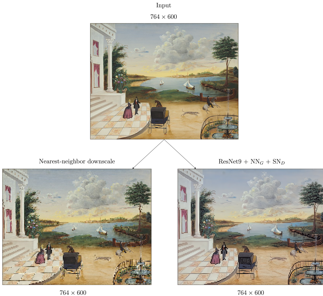
Figure 7.7.: A comparison of the ResNet model and nearest-neighbor interpolation on a input painting of size 764 \times 600 .
