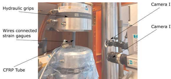
Fig. 4. Experimental setup used in the presented research equipped with a camera I used for sample monitoring, camera II as a part of used DIC system, and strain gauges.
