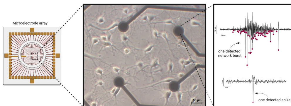
Figure 7. Microelectrode arrays. Schematic of a microelectrode array with an inset of a cell culture showing neurons widespread around the electrodes (black circles). The electrodes will capture spontaneously evoked extracellular network activity from the neurons which can be captured as network bursts (top) and single spikes (bottom). Figure created in BioRender.com.
