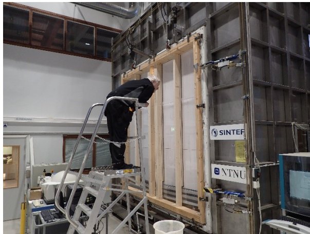
FIGURE 1. The test wall installed in the driving rain apparatus undergoing visual inspection for rain penetration. The rear of the wall is facing to the laboratory.
