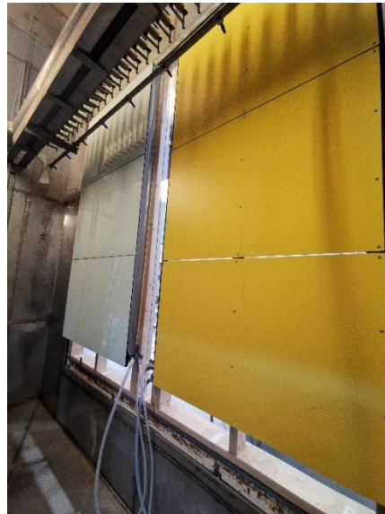
FIGURE 4. Test wall observed from the inside of the driving rain cabinet. The water spray nozzles can be observed at the top.
