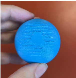
(a) Supports removed with pliers.
