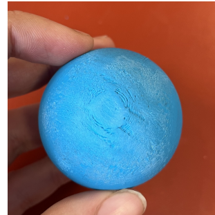
(b) Rest of supports sanded down.
