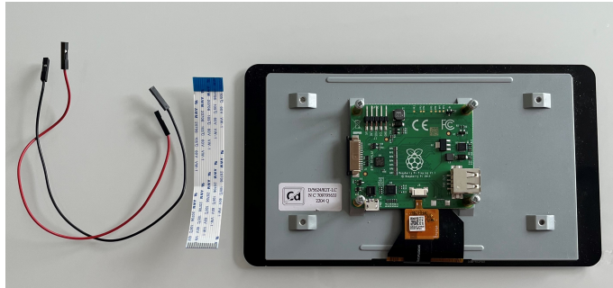
Figure 3.6.: 7" Raspberry Pi touch Display with DSI cable and wires.
