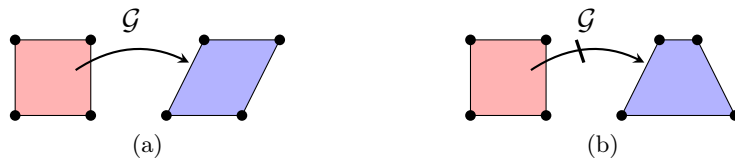
Figure 7: Illustration of an affine mapping \mathcal{G} : \hat{T} \mapsto T versus a non-affine transformation. The left figure preserves parallel lines before and after the transformation, indicating an affine transformation. However, the right figure does not maintain parallelism, making it a non-affine transformation.
