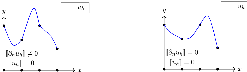
Figure 2: Illustration of global C^0 continuous elements (left) and global C^1 elements (right) in 1 dimension. Here, u_h is a discrete solution, where the jump between the elements is denoted as [[u_h]] = u_+ - u_- .
