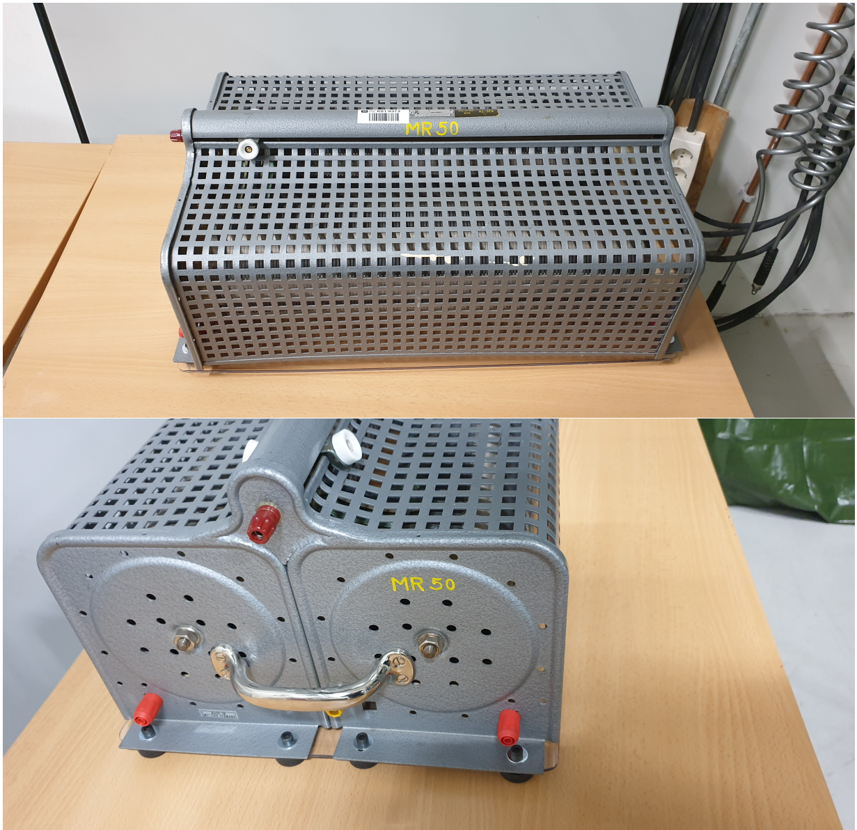
Figure B.6: Picture of the single phase resistance that was used as parallel branch load during testing. The resistance of the load could be adjusted from 5\Omega to 25\Omega
