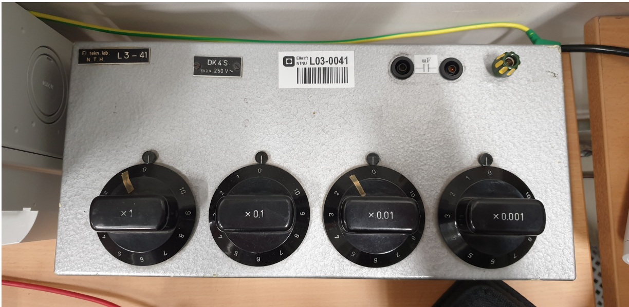
Figure B.7: Picture of the adjustable capacitance that was used as parallel capacitance during testing. The capacitance was adjustable in the range of 1\text{ nF} to 11.11\mu\text{F}
