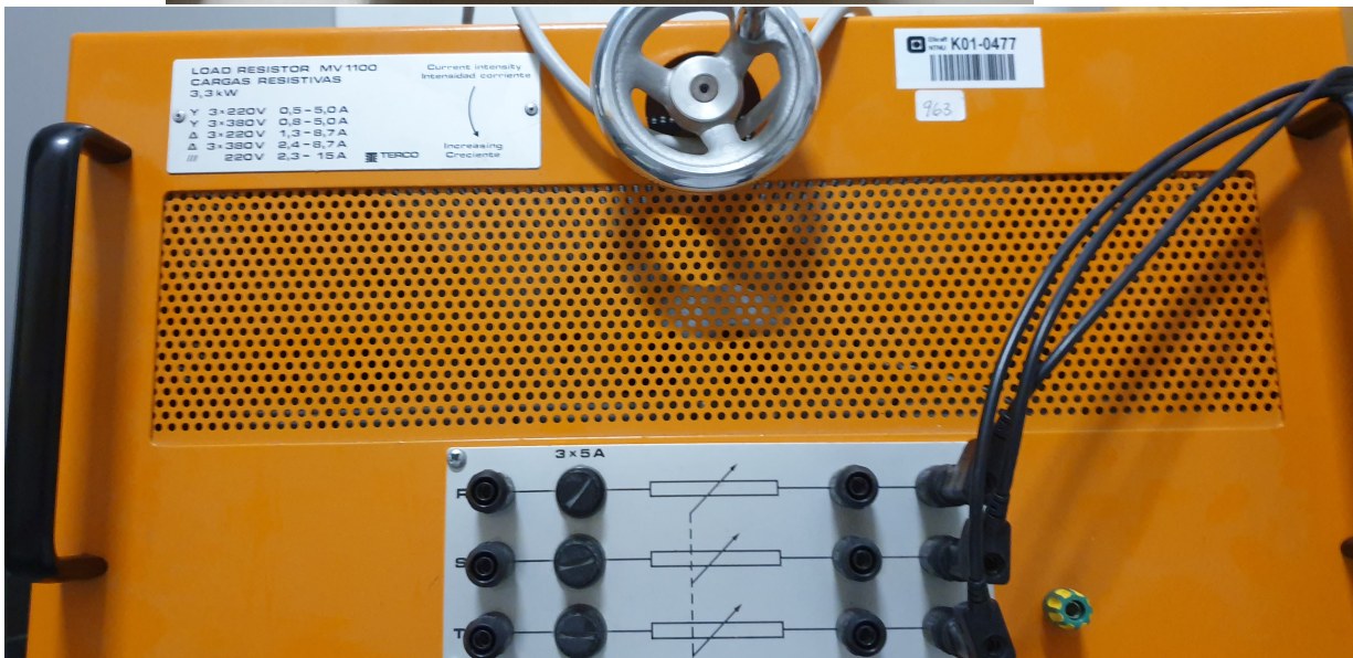
Figure B.5: Picture of the three phase load that was used as arc branch load. An adjustable load was used so the arcing current could be adjusted from <1.0\text{A} to 15\text{A} . Each phase of the load had a resistance that could be adjusted from 100\Omega to 14\Omega with the possibility of parallel or series connecting as needed
