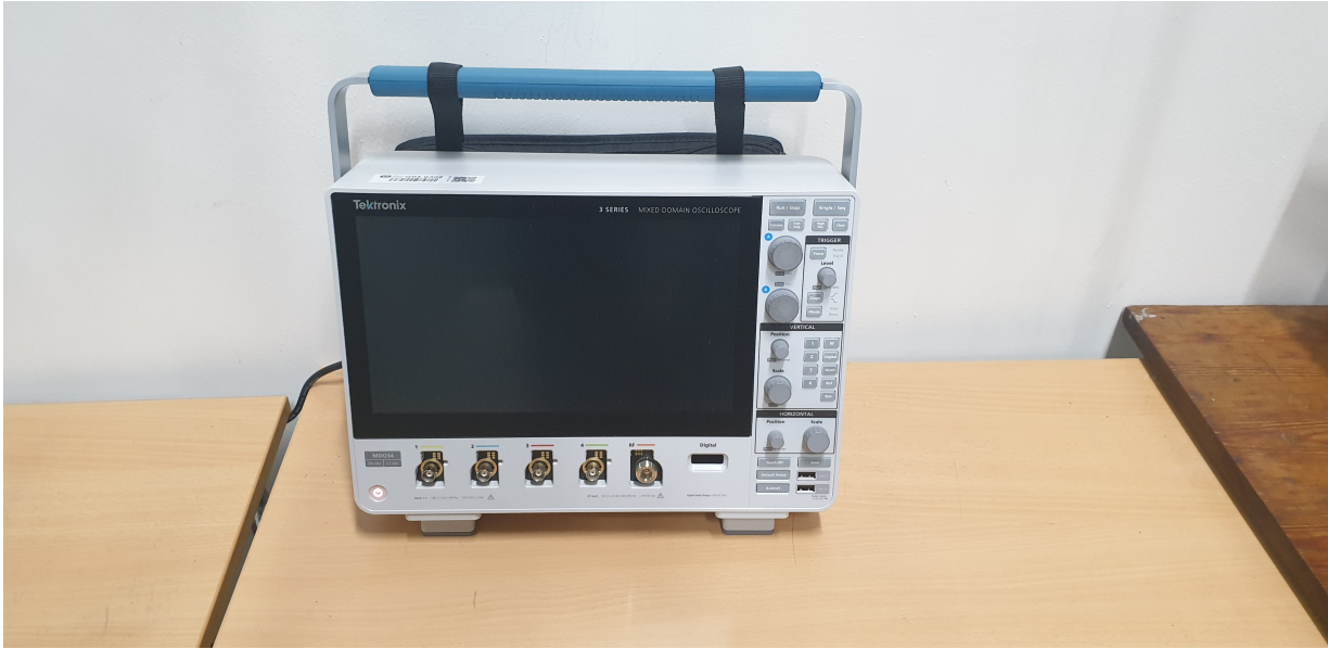
Figure B.3: Picture of the Tektronix MDO34 mixed domain oscilloscope used in the tests. The maximum sampling rate of this oscilloscope was 2.5 GS /s, with a bandwidth of 200MHz and a maximum record length of 10 million samples
