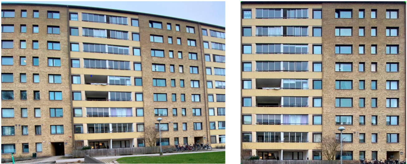
Figure 8. Façade images before and after barrel/pincushion and perspective distortion correction.
