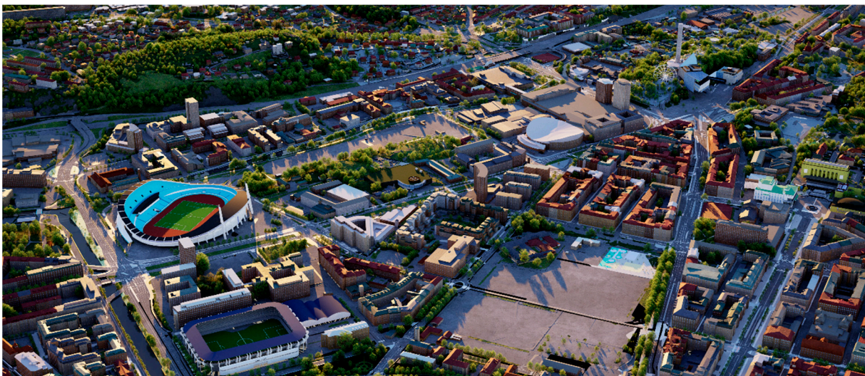
Figure 2. Part of the current 3D model in Gothenburg. The model is constructed by parametric design, but does not yet have any connection to external databases within the city.
