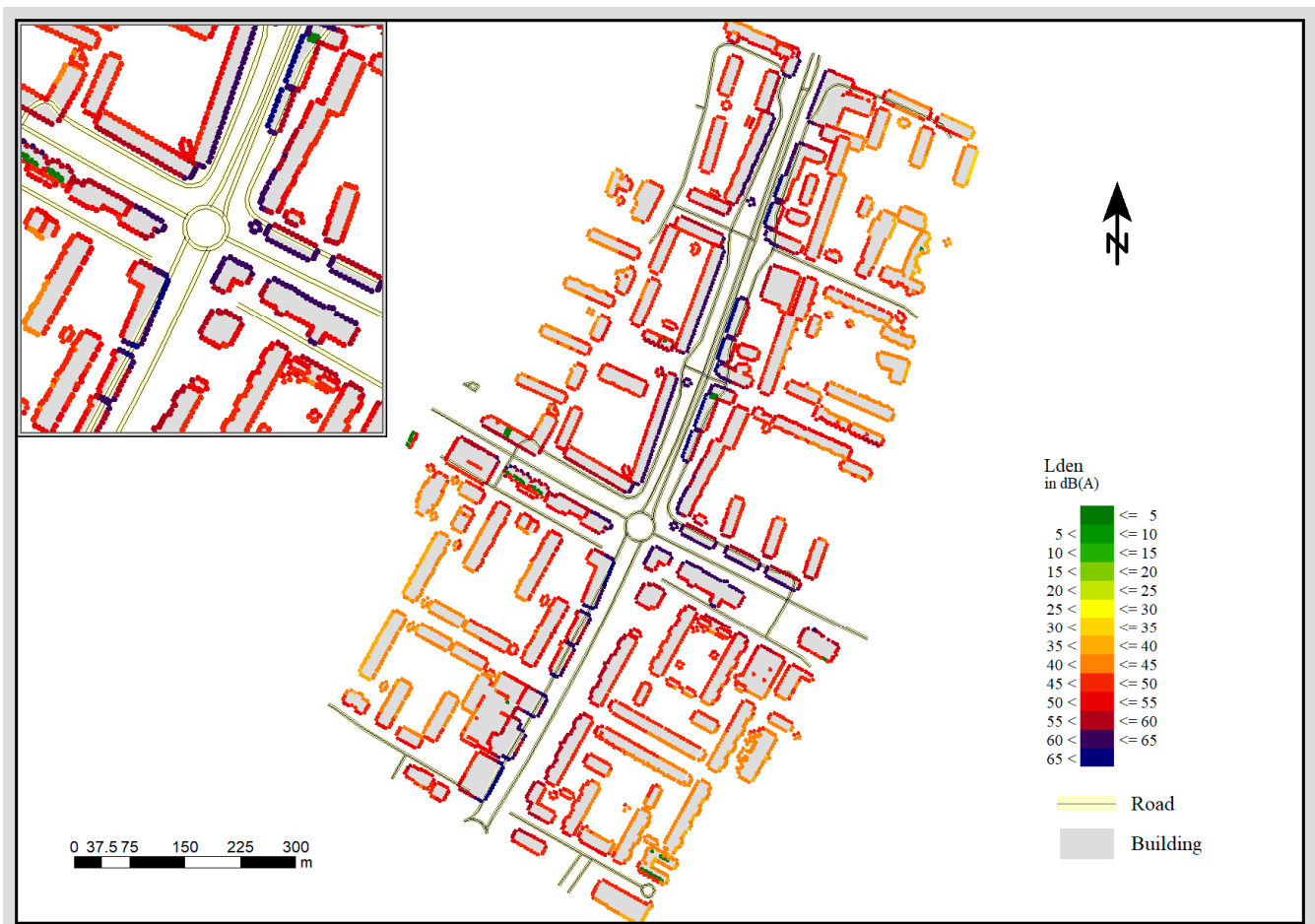
Figure 17. Result of noise simulations in the Lorensborg–Bellevue area in Malmö. The simulations were performed in SoundPlan in accordance with the CNOSSOS-EU model. Lden is a descriptor of noise level over a whole day, with a penalty of 5 dB(A) for evening noise (19.00–23.00) and a penalty of 10 dB(A) for night-time noise (23.00–7.00). It should be noted that this simulation was performed with some planned buildings included; therefore, there is some overlap between current roads and building objects.
