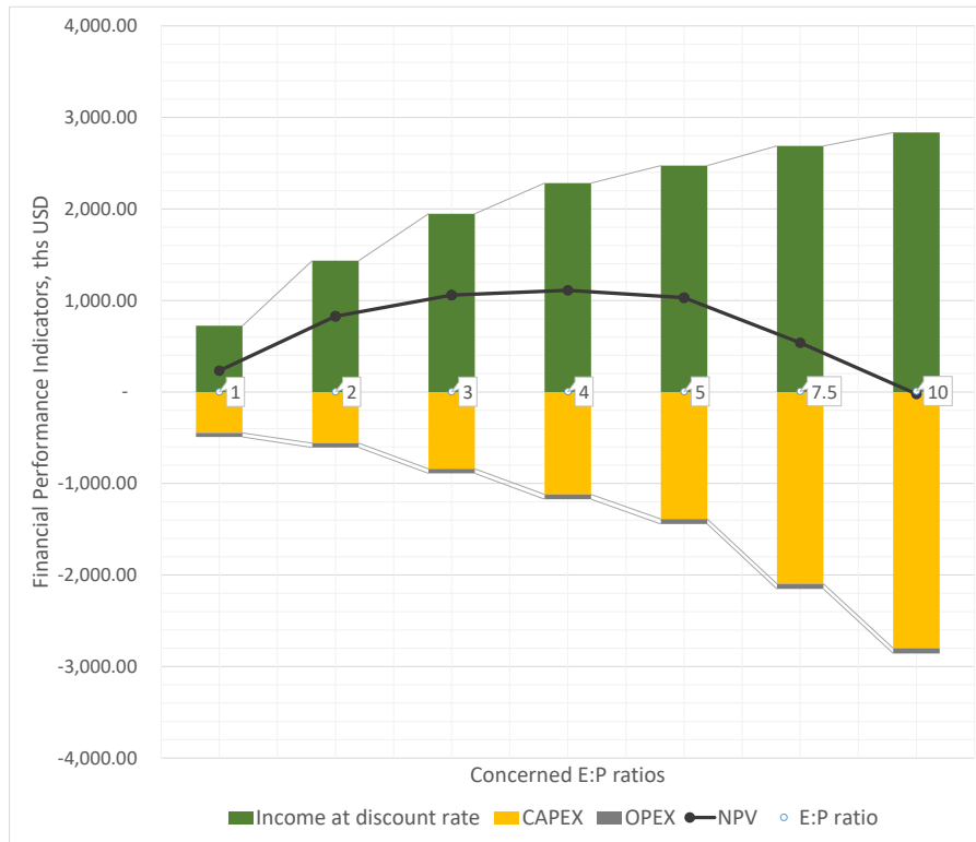
Figure 5.8: Comparison of NPV at the end of a lifetime of BESS in Elspot market, ths USD.
