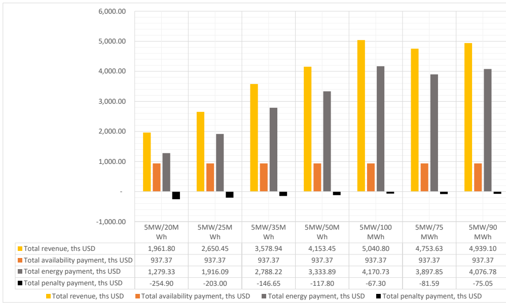
Figure 5.27: Comparison of annual revenue streams of CAES in mFRR market, ths USD.
