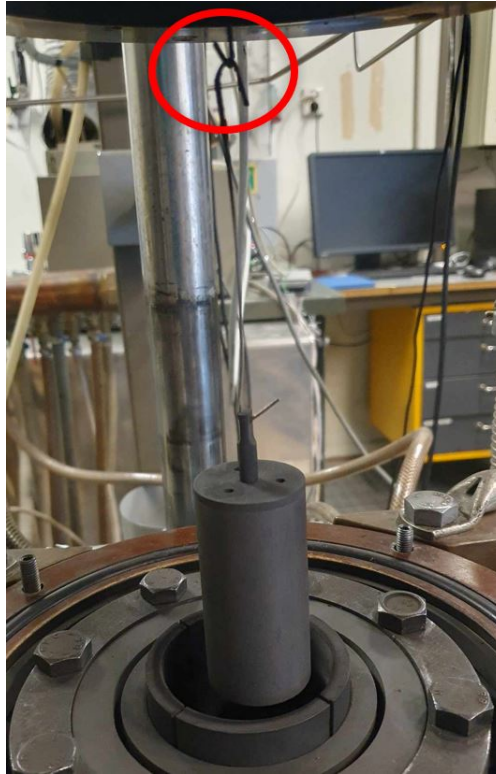
Figure 3.4: Graphite crucible suspended in the TG furnace. The connection between the two Mo wires is marked with red circle.
