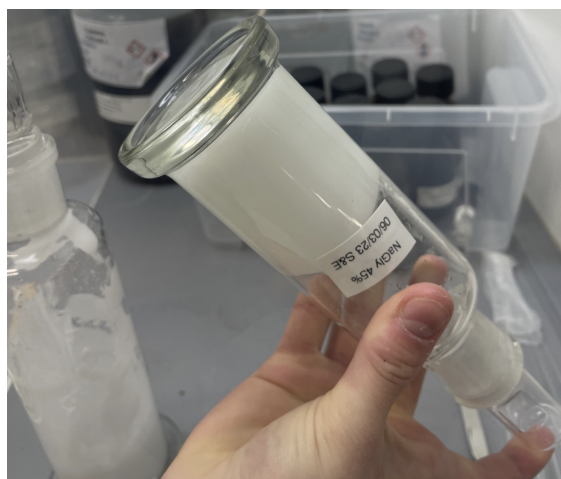
Figure 23: 45 wt% NaGly solution, 24 hours after ended experiment
