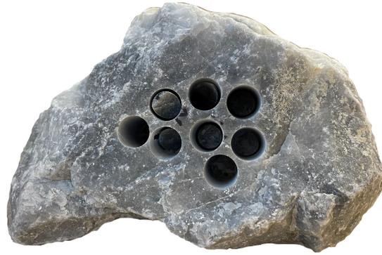
Figure 3.2: Image of the quartz block used to extract and produce quartz substrate disk for wetting experiments.
