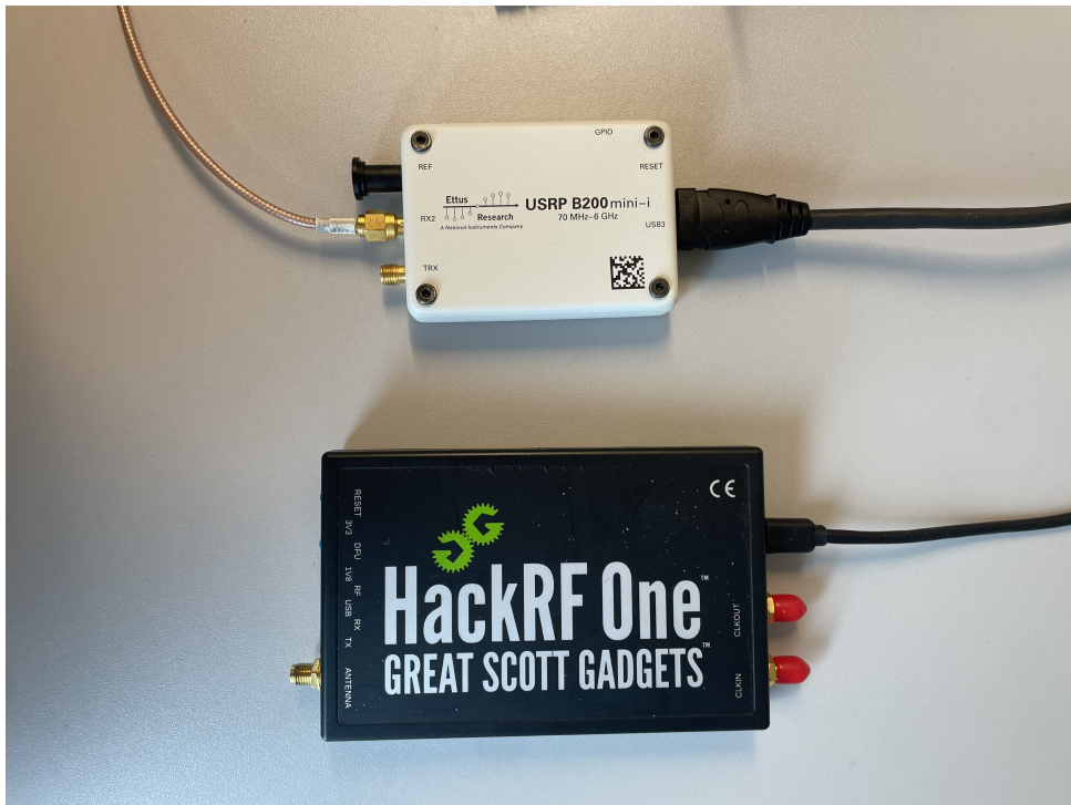
Figure 5.1: USRP and HackRF One used in the experiment
