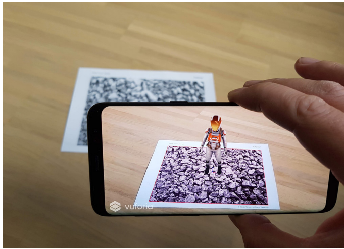
Figure 14: Anchoring with a QR-code, using the software Vuforia [66], with a phone acting as a VST mixed-reality device. Source: [76]
