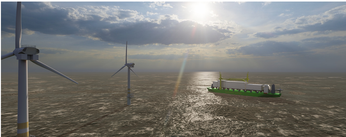
Figure 3.15: Floating ammonia production unit concept by SwitchH2 and BW Offshore (DNV 2023a).
