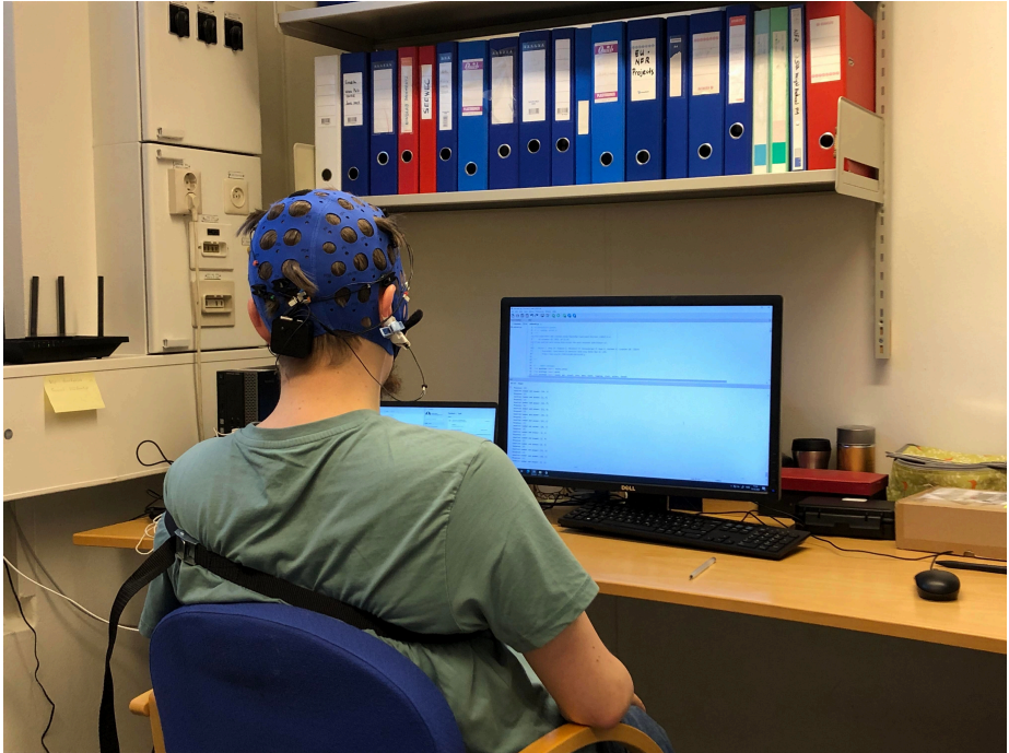
Figure 3.1: A photograph taken during a recording session. The participant is seen wearing the Mentalab Explore EEG device, identifiable by the blue cap. The Eko DUO PCG device is securely fastened to the participant's chest using the buckle strap shown on the participant's back. The monitor placed in front of the participant is used to display the arithmetic questions.
