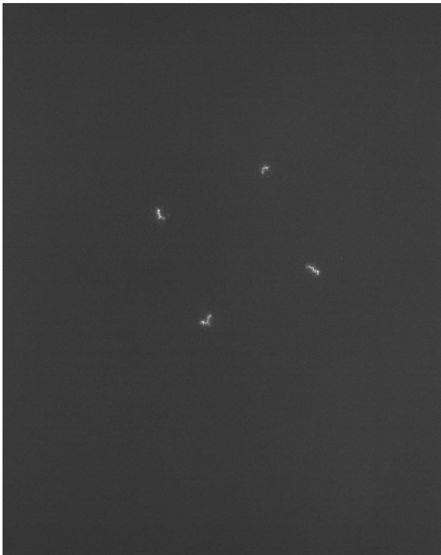
Figure 38: Picture of the substrate surface with bipolar voltage at 11\text{ kV}_{peak} in Nytro 10XN with a camera frequency of 480 Hz: Picture number 7 (in Figure 30).
