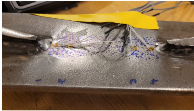
Figure 26: Strain gauges placed on a test specimen near the weld toes (Mosbron 2022)
