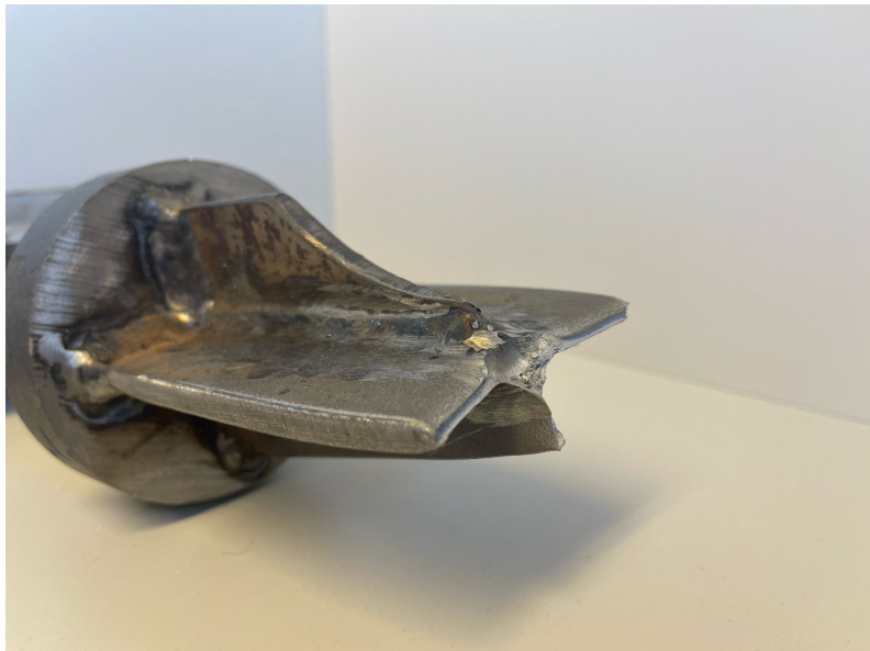
Figure 40: The fatigue crack in the test specimen after Mosbron's fatigue test
