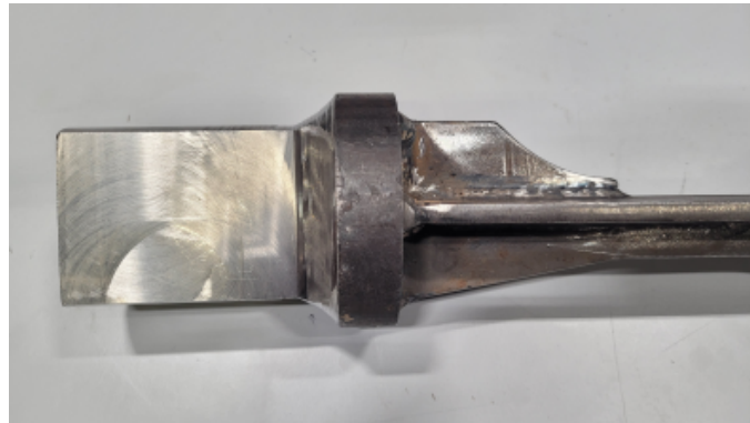
Figure 25: The grip section on the test specimen (Mosbron 2022)
