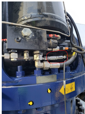
Figure 16: The pressure transducer is coupled to an entrance on the block on the main cylinder of the crane.
