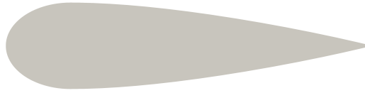
Figure 3.4: 3:2 elliptic nose with NACA 0020 tail
