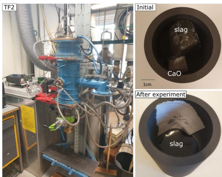
Figure 87 A picture of the graphite tube furnace, TF2 (left) and the crucible setup (right). The top right picture is the initial crucible with CaO and SiO 2 -CaO-Al 2 O 3 slag and the bottom right shows the same crucible after heating to 1600 °C.
