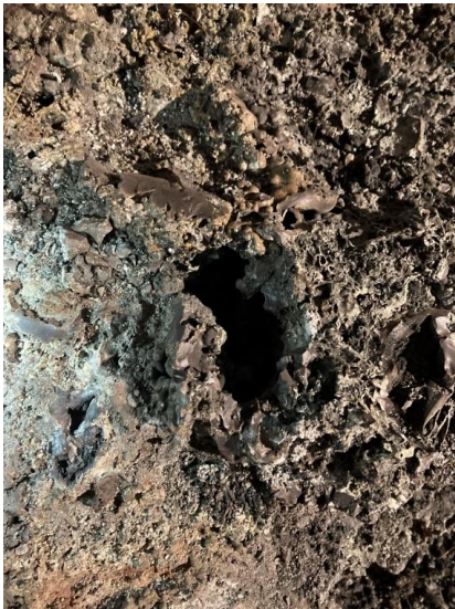
Figure 202 Picture of sample CPO1101 and what appeared to be gas channels where SiO and CO gas have found its way through the hard and compact charge.
