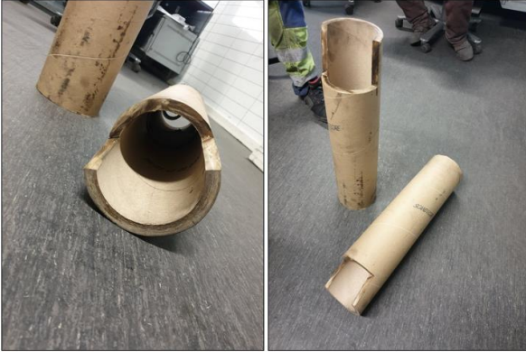
Figure 25 Equipment used for sampling of tapped slag. The compressed paperboard is designed to be used as a “spoon” to dig out slag from the tap-hole.
