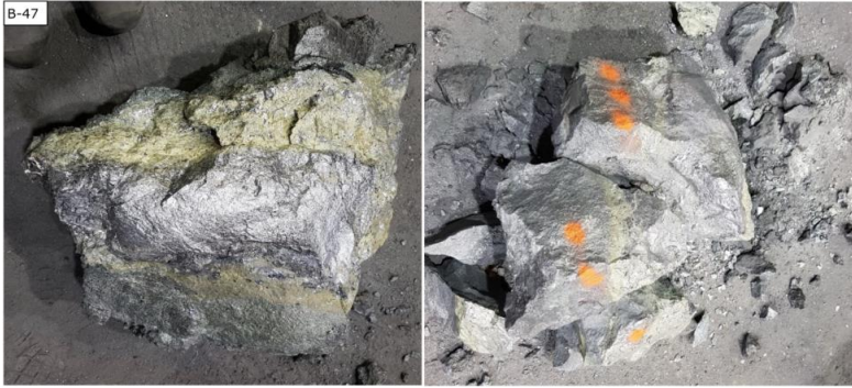
Figure 186 The left picture shows the collected sample at the plant, B-47 from tap-hole 7, and right picture shows the sample crushed into three pieces. The pieces were marked with One, two or three orange dots.
