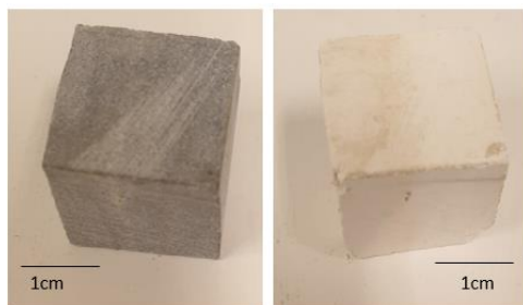
Figure 86 Picture of the original limestone to the left, and after calcination 1h at 1000 °C to the right.
