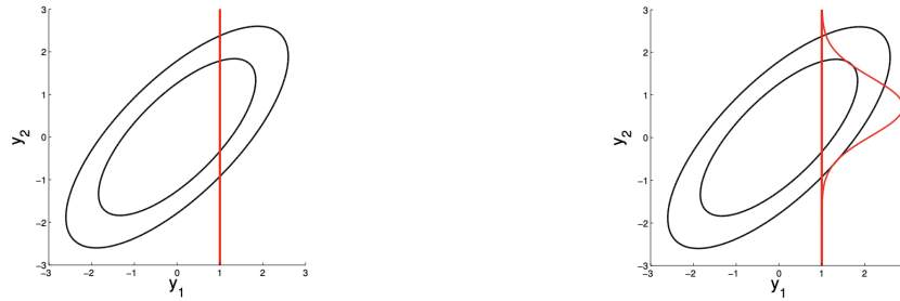
(a) A variable y_1 fixed to a single value, allowing (b) Probability density of the variable y_2 computed based on the fixed variable y_1 .
