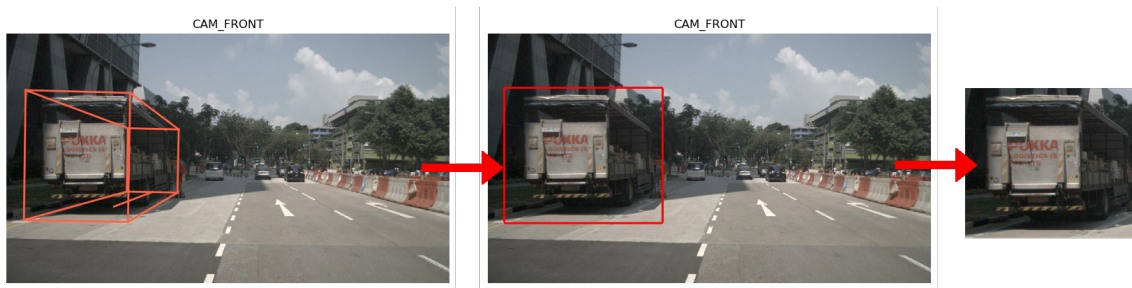
Figure 4.3: An image sequence showing the 3D to 2d pipeline. The initial 3D bounding box is converted to 2d, and the edges of the bounding boxes are then used to crop the image to only contain that object.
