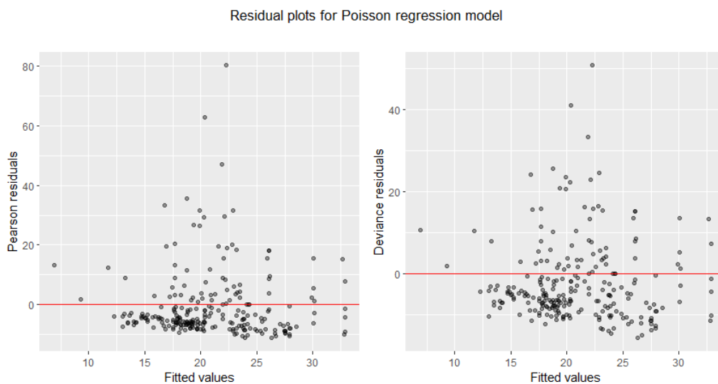
Figure 12: Plot of Pearson and deviance residuals against fitted values from the Poisson regression model. To visualize overlapping, the data points are partially transparent. The data points with the lightest black colour indicate a single point, while a darker black colour indicates overlapping points.
