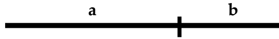
Figure 3.1: A line segment divided by the golden ratio. The total line length divided by the long part is equal to the long part divided by the short part. Both ratios are equal to the golden ratio \phi .
